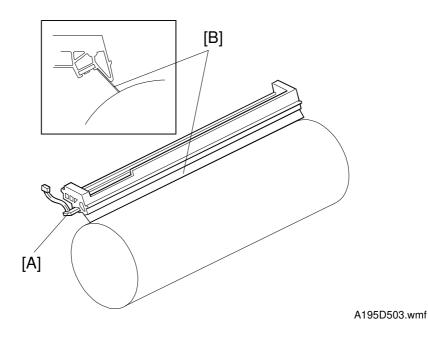
In preparation for the next copy cycle, light from the quenching lamp [A] neutralizes any charge remaining on the drum.
