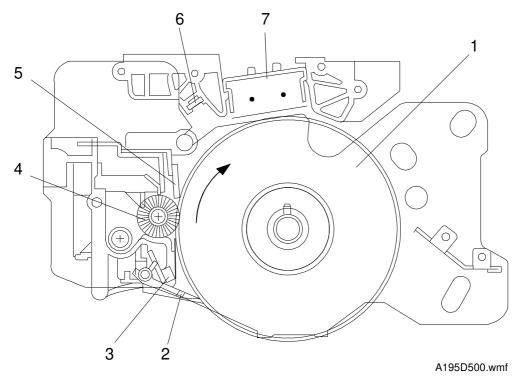
The drum unit consists of the components shown in the above illustration. An organic photoconductor (OPC) drum (diameter: 100 mm) is used in this model.
