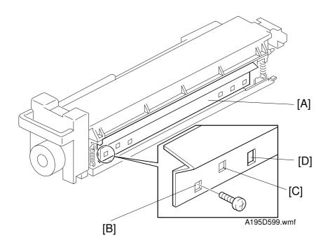
The entrance guide [A] for this machine has three holes on each side to adjust for thick or thin paper. Normally, the outer screw hole [B] on each side is used.
