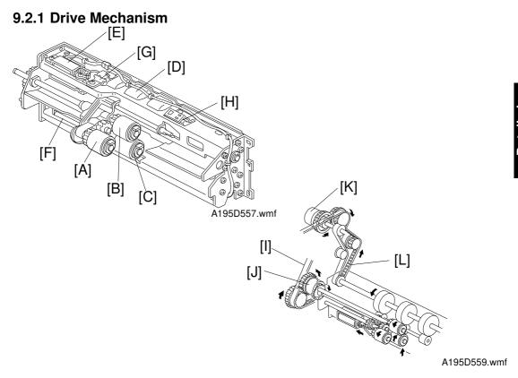
The paper feed unit consists of a pick-up roller [A], feed roller [B], separation roller [C], relay roller [D], pick-up solenoid [E], separation solenoid [F], paper upper limit sensor [G], and paper end sensor [H].
