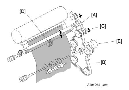
Main motor rotation is transmitted to the registration clutch gear [A] (located on the lower registration roller shaft) through the timing belt [B] and the relay gear [C].
