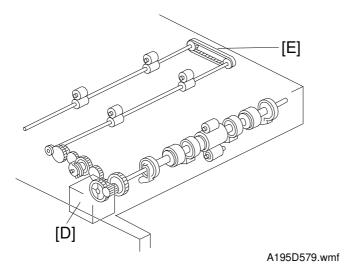
The main motor [A] drives the transport rollers [B] through the timing belts [C]. All rollers in the duplex tray are driven by the duplex feed motor [D] through a series of gears and a timing belt [E]. Helical gears are used to reduce noise.
