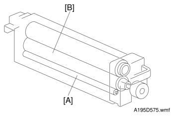
The cleaning roller [A] is always in contact with the pressure roller [B]. It collects toner and paper dust adhering to the surface of the pressure roller. This is because the cleaning roller is made of metal and collects adhering matter more easily than the pressure roller (which has a teflon coating).
