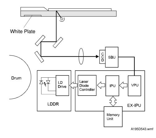
The CCD generates an analog video signal. The SBU (Sensor Board Unit) then sends the analog video signal to the EX-IPU (Extended Image Processing Unit) board.
