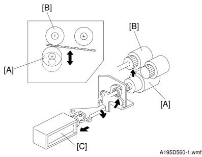
This FRR mechanism uses a separation roller release system. The separation roller [A] is normally away from the feed roller [B]. When the paper feed station has been selected and the Start key is pressed, the separation solenoid [C] moves the separation roller into contact with the feed roller.
