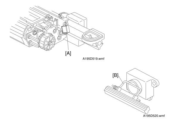
The toner end sensor [A] (which is a piezoelectric sensor) detects whether there is sufficient toner in the toner supply unit or not.
