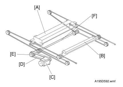
A five-phase stepper motor is used to drive the scanner. The 1st and 2nd scanners [A,B] are driven by this scanner drive motor [C] through the timing belt [D], scanner drive pulley [E], scanner drive shaft [F], and two scanner wires.
