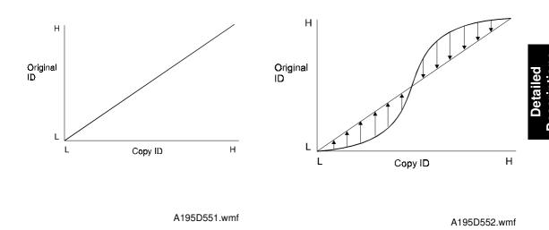
This corrects the response of the CCD and the characteristics of the printer (i.e., the characteristics of the drum, laser diode, and lenses) to the various shades in the gray scale from black to white. The relationship between original ID and copy ID should be constant as shown in the diagram on the left. However, in reality, it is more like that shown in the diagram on the right. Gamma correction corrects the data for this deviation.
