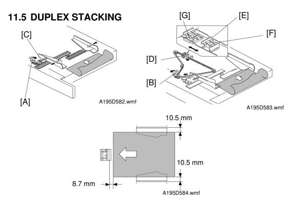
There are two motors for driving the fences. The side jogger fences are driven by the side fence jogger motor [A]. The end jogger fence is driven by the end fence jogger motor [B]. Using two separate motors for the side and end fences allows the duplex tray to handle all paper sizes from A3/11" x 17" to A5/ 81/2" x 51/2" sideways.
