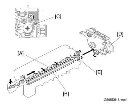
Inside the toner supply unit are the transport screw [A] and the toner supply roller [B]. As the grooves in the toner supply roller turn past the slit [C], toner falls into the development unit.
