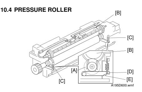
The pressure roller [A] is made of silicone rubber with a teflon tube coating. The pressure springs [C] constantly apply pressure between the hot roller [B] and the pressure roller.
