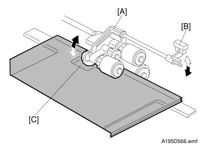
If there is some paper in the paper tray, the paper end feeler [A] is raised by the paper stack and the paper end sensor [B] is deactivated.
