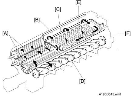
This copier uses a standard cross-mixing mechanism to keep the toner and developer evenly mixed. It also helps agitate the developer to prevent developer clumps from forming and helps create the triboelectric charge.
