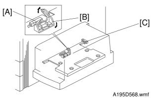
The LCT paper end sensor [A] is just under the LCT bottom plate.
