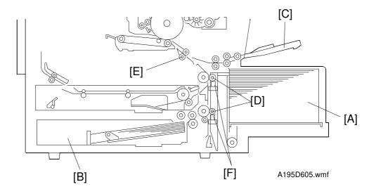
This model has three paper feed stations: the large capacity tray feed station [A], the paper tray feed station [B], and the by-pass feed station [C].
