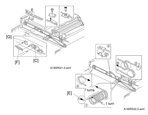
26. Wind the left side of the wire counterclockwise towards the front side (1 turn) and the right side of the wire counterclockwise towards the rear (7 turns) as shown.
