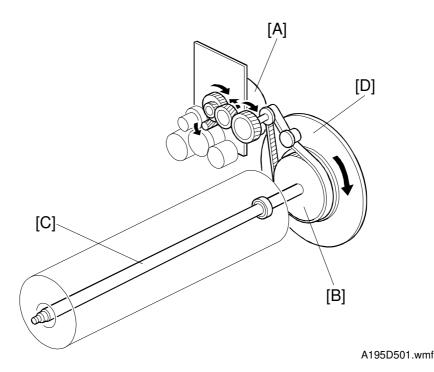
The drive from the main motor [A] is transmitted to the drum through a series of gears, a timing belt, the drum drive pulley [B], and the drum shaft [C]. The main motor has a drive controller, which outputs a motor lock signal when the rotation speed is out of the specified range.
