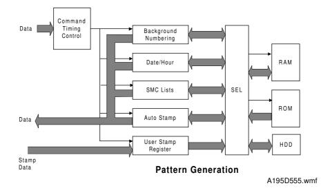
The pattern generation circuit consists of the pattern generation circuit in the GA4 IC, RAM, ROM and Hard Disk. The pattern generation circuit has the following functions.
