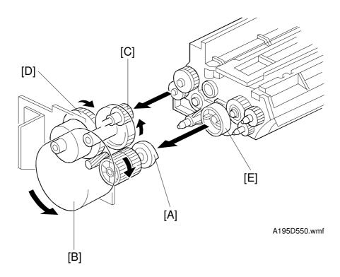
The development drive motor [B] rotates the development drive gear [A], which drives the gears in the development unit.
