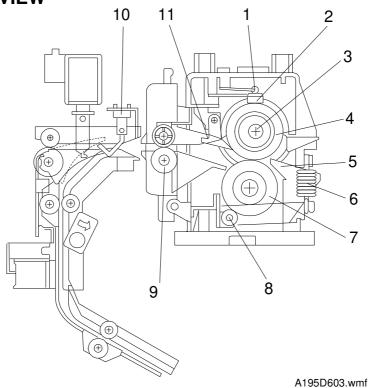
The fusing unit consists of the following parts:
