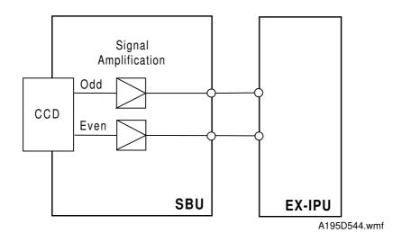
The CCD converts the light reflected from the original into an analog signal. The CCD line has 5,000 pixels and the resolution is 400 dpi (15.7 lines/mm).
