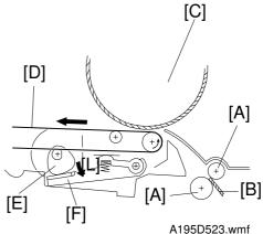
(2) Before the leading edge of the paper reaches the gap between the transfer belt and the drum, the transfer belt lift clutch [G] rotates half of a complete rotation to release the lift lever. Then, the transfer belt is pushed up as a result of spring pressure. The contact width [H] is about 12 mm.
