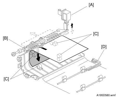
The junction gate solenoid [A] is energized 1.1 seconds after the registration clutch has been turned on. Then, the junction gate [B] rotates upwards to direct the copy paper to the duplex turn guide. The junction gate solenoid stays on until the first side copies are stacked in the duplex tray.
