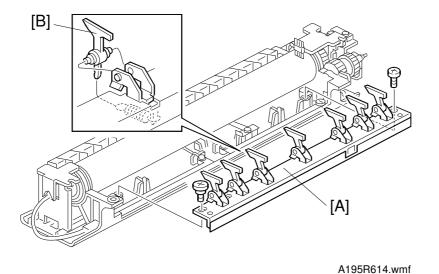
1. Remove the fusing unit. (See Fusing Unit Removal.)
