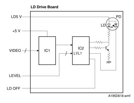
Even if a constant electric current is applied to the laser diode, the intensity of the output light changes with the temperature. The intensity of the output decreases as the temperature increases.
