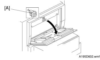
The by-pass feed table switch [A] detects when the by-pass feed table is opened. Then the CPU turns on the by-pass feed indicator on the operation panel.
