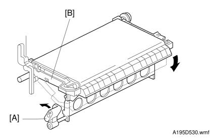
When the transfer belt unit release lever "A1" [A] is rotated counterclockwise, the transfer belt unit [B] is released, allowing it to drop. This mechanism allows easy paper jam recovery and easy maintenance of the transfer belt unit.
