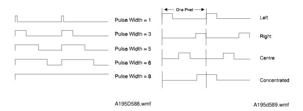
The width of the laser pulse for each pixel has 8 settings (see the diagram on the left at the bottom of the previous page).
