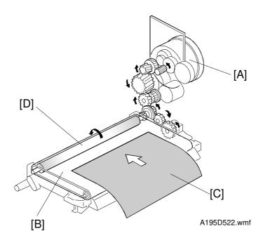
The main motor [A] drives the transfer belt [B] through a series of gears. Since the transfer belt attracts the paper [C] electrostatically, a transport fan is not required.
