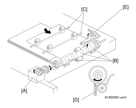
The duplex feed motor [A] starts turning 500 ms after the leading edge of the paper activates the fusing exit sensor. This motor drives the duplex feed rollers [B] and the duplex transport rollers [C]. The copy paper from the turn guide is directed to the duplex tray through these rollers.
