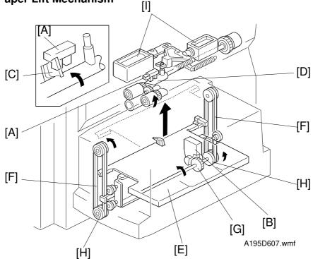
The LCT upper limit sensor [A] above the paper feed upper guide plate controls the LCT lift motor [B]. The actuator [C] for the sensor is on the pick-up roller shaft [D]. The LCT lift motor drives the LCT bottom plate [E] which is attached to the timing belts [F] through the helical gear [G] and drive pulleys [H].
