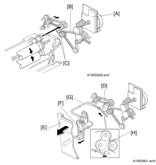
The main motor [A] drives the fusing unit through a timing belt [B] and some gears [C].
