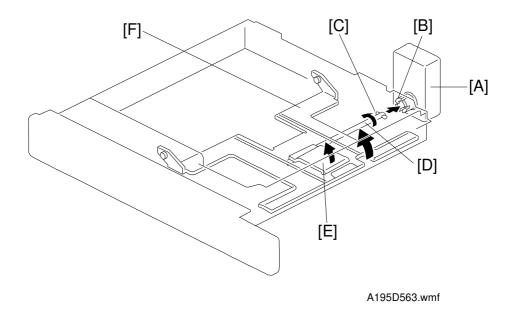
The tray switch detects when the tray is placed in the machine. When the machine detects that the paper tray is in the machine, the tray lift motor [A] rotates and the coupling gear [B] on the tray lift motor engages the pin [C] on the lift arm shaft [D]. Then the tray lift arm [E] lifts the tray bottom plate [F].
