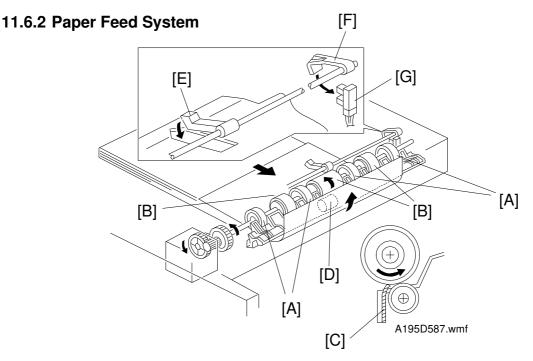
While paper is being stacked in the duplex tray, the paper flatteners [A] correct curl at the leading edge of the paper.
