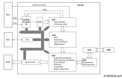
The EX-IPU uses seven LSIs and a hard disk to process the video data. These LSIs have the following functions.
