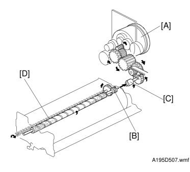
Drive from the main motor [A] is transmitted to the cleaning brush gear [B] via a series of gears, a timing belt, and the joint gear [C]. The cleaning brush gear then transmits the drive to the toner collection coil [D].
