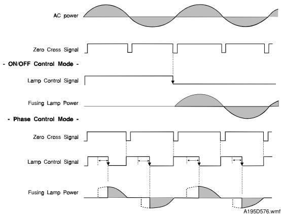
In on/off control mode, the ac drive board supplies full ac power to the fusing lamp.
