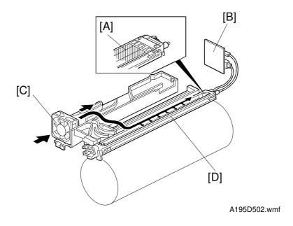
This copier uses a double corona wire (single loop type) scorotron system for charging the drum.
