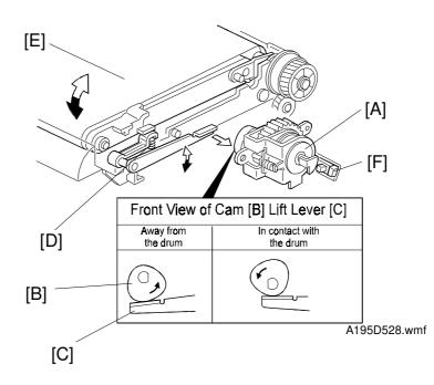
The transfer belt lift clutch [A] (a half turn clutch) located on the back of the copier turns on and the cam [B] rotates half of a complete rotation. The lift lever [C], riding on the cam is lifted up and the spring [D] pushes up the transfer belt [E] for it to contact the drum.
