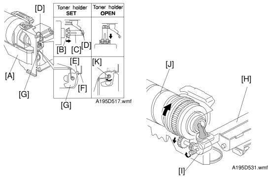
When a toner cartridge is placed on the holder unit [A] and pushed back in completely, the following procedures are performed automatically to allow toner to be supplied to the toner supply unit.
