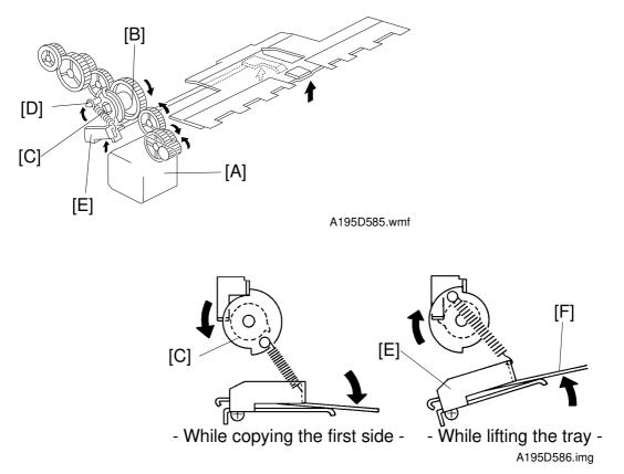
After the first side copies have been made, the duplex feed motor [A] changes direction, and the cam clutch gear [B] lifts up the duplex bottom plate through a series of gears.
