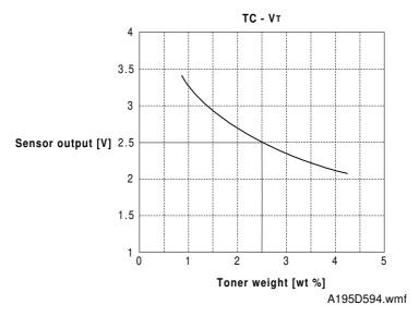
Developer consists of carrier particles (ferrite) and toner particles (resin and pigment). Inside the development unit, developer passes through a magnetic field created by coils inside the toner density sensor. When the toner concentration changes, the voltage output by the sensor changes accordingly.
