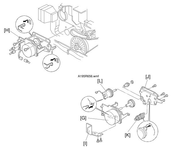
9. Remove the fan motor [G]. (2 screw, 1 connector.)
