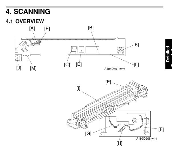
An image of the original illuminated by the exposure lamp (a halogen lamp in this model) [A] is reflected onto a CCD (charge coupled device) [B] via the 1st, 2nd, 3rd mirrors, green filter [C], and lens [D].
