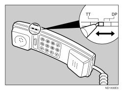
The switch on the handset should be in the appropriate position-TT (Tone Dialing) or DP (Pulse Dialing).
