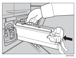
Push the unit into the machine until it clicks into place.
