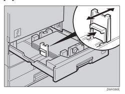
Adjust the tray size with the paper size selector to the new paper size.
