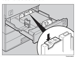
While pressing the release lever, adjust the back fence to the new paper size.
