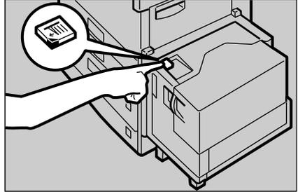
**2** After the **Down** key stops blinking, open the cover.
