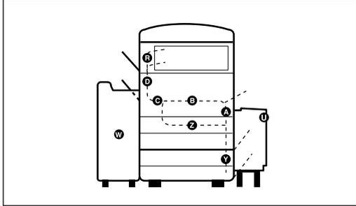
**⚠ CAUTION** When removing misfed paper, do not touch the fusing section because it could be very hot.
