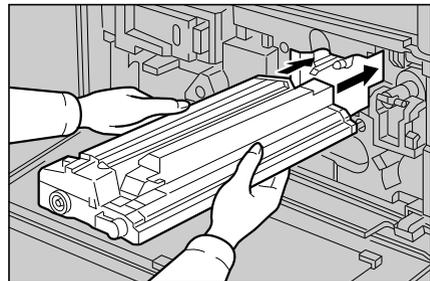
**11** Push the new PCU in until the release lever lock.
