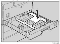
While pressing the levers on the rear guides, slide the rear guides
