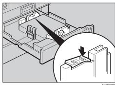
While pressing the release levers on the front and rear guides, slide
