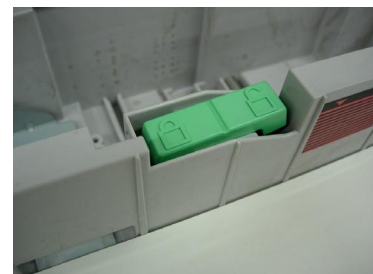
Side fence lock is locked .
