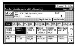
The selected folder is highlighted and also is displayed in the destination field at the top of the screen.
