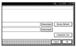
A connection test is performed to check whether the specified shared folder exists.
