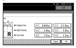
Make sure that the area specified in step 4 (X3 and Y3) is shown in the [Custom Size] field, and then press [OK].
