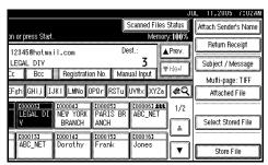
2 Enter the five digit registration number that has been assigned to a destination folder using the number keys.
