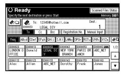
The selected destination is highlighted and also displayed in the destination field at the top of the screen.
