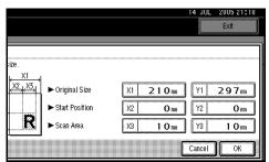
**3** Enter the scan starting point in relation to the standard scan starting point.
