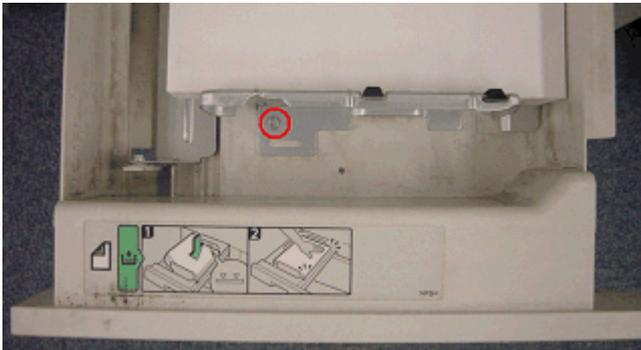
2. Clean the attachment area for the new tape (red area shown in the photo) with alcohol.
