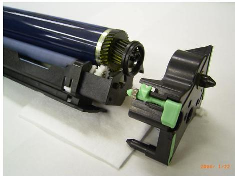
3. Hold the drum at both ends as shown, then slide it in the direction of the arrow **until the outer gear clears the PCU frame** (see the second photo, at the top of the next page).
