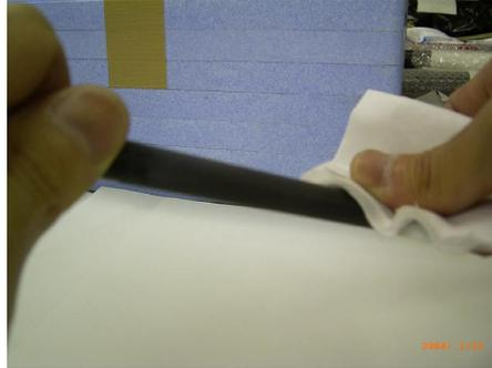
11. Hold the charge roller **by the tape-covered edges only**, and then attach parts B, C and D.
