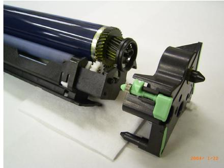
3. Hold the drum at both ends as shown, then slide it in the direction of the arrow **until the outer gear clears the PCU frame** (see the second photo).
