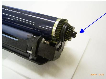
Slide the drum until this outer gear clears the PCU frame, as shown.
