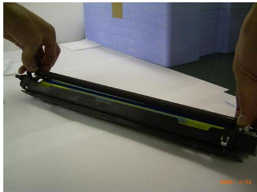
8. Put the charge roller on a cloth-covered surface.
