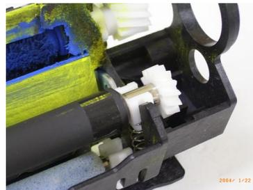
13. Hold the drum at both ends, and then put the drum gear inside the hole in the frame.
