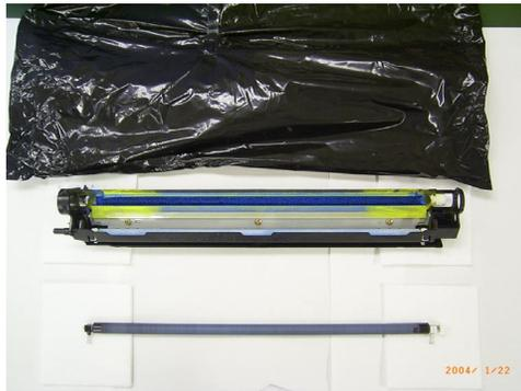
9. Hold the charge roller **by the tape-covered edges only**, and then remove parts B, C, and D.
