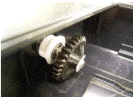
5. Put back the bearing so that the flat sides of the bearing are parallel with the ribs (see the left photo).
