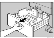
2 Align the paper and load it in the tray with the print side up.
