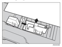
8 Confirm that the paper is fixed in place, and then lock the side guides.
