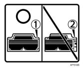
Make sure the toner cartridge is not misaligned to the left (2). If it is, carefully lift and move the cartridge to the right so it is located at (1).
