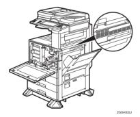
When you open the internal cover of the duplex unit (right side of the machine), you can see the holes in the upper surface of the development unit (the part with the warning label). Normally, from here you will be able to see the orange heat roller. If you can see paper in this area, contact your service representative.
