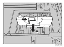
Pinching both sides of the end guide (①), move the end guide in the direction of the arrow (②) to open it.
