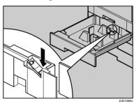
5 While pressing the release lever, adjust the side guides to the paper size.
