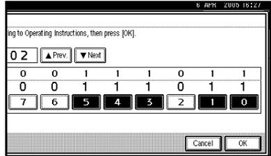
When the bit number is pressed, the current value switches between 1 and 0.
