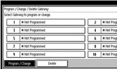
When registering a new gateway, press **[\*Not Programmed]**.
