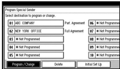
When programming a new Special Sender, press **[\*Not Programmed]**.
