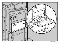
Insert the paper with the side you want to copy facing down until you hear the beep, and align the paper guide to the paper size.
