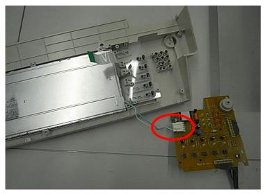
5. Remove the LCD and the touch panel from the operation panel (screw x 4)
