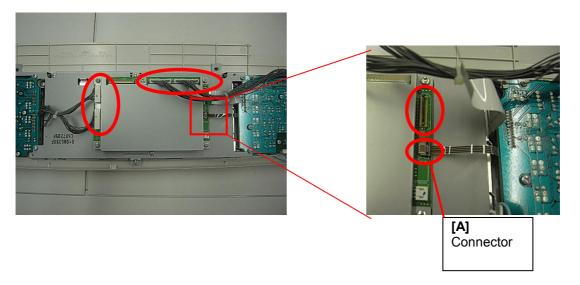
3. Remove the operation panel bracket (screw x 8).
