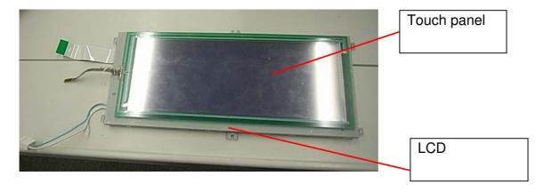
7. Attach the new touch panel (P/N **H3106173**) to the LCD. **Important:** Only replace the touch panel. Do not replace the LCD.
