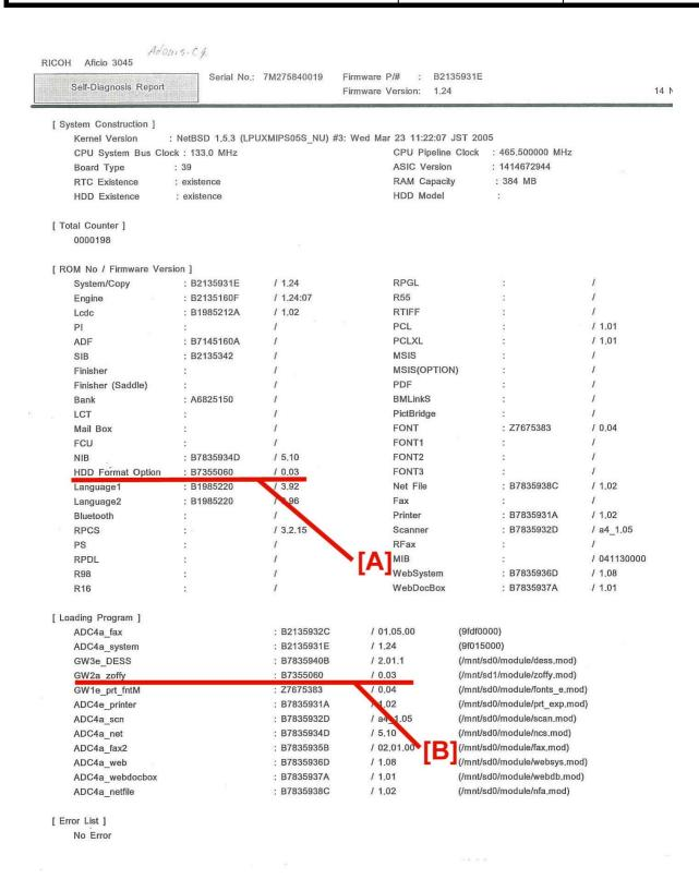
**Note:** This photograph is just an example for when **Type D** is installed. Because the numbers in **[A]** are the same as the numbers in **[B]**, the unit was installed correctly.
