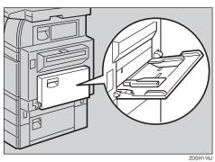
2 Insert the paper with the side you want to copy facing down until you hear the beep, and then align the paper guide to the paper size.
