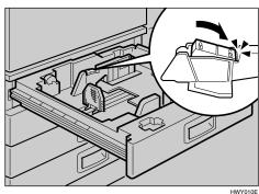
4 While pressing the release lever, adjust the side fences.
