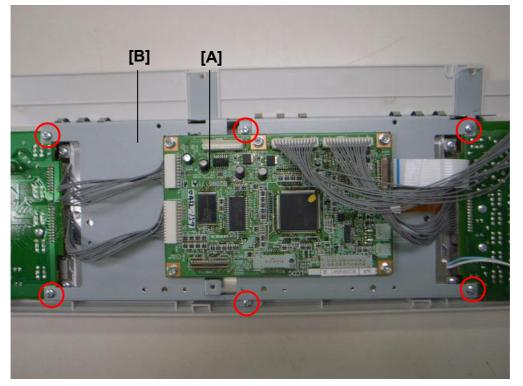
3. Remove the 4 screws from the LCD (circled below in red). Then, detach the LCD from the operation panel as shown.
