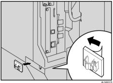
2. Connect the USB cable to the machine.
