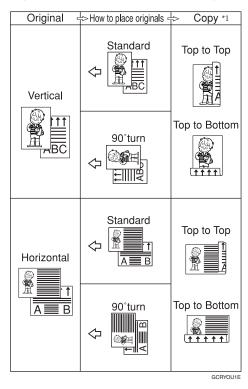
\*1 This table shows the orientation of images on the front and back of copies, not the orientation of delivered copies.
