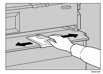
**5** Insert the paper in the bypass tray, copy side up.
