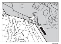
Reattach the duplex feed unit using the screw removed in step 4.
