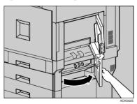
2 Move the blue lever (A) up and down to remove the misfed paper.
