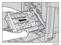
**2** Place the duplex feed unit gently on the floor. Slowly open it, and remove the misfed paper.
