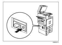
6 Confirm that the earth leakage breaker switch moves to the off position.
