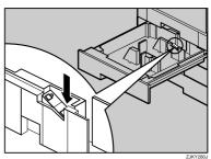
While pressing the release lever, adjust the side guides to the paper size.
