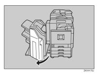
2 Pull out the punch waste box, and then remove punch waste.
