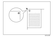
☐ When the ADF is installed, make sure to set the test pattern on the exposure glass, and then 2 or 3 white sheets, same size as the test pattern, above the test pattern.
