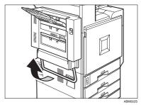
Using the tip of a ball-point pen, press the test button of the earth leakage breaker.
