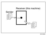
Normally this machine receives messages by Immediate Reception. But Memory Reception is used when "Combine 2 Originals", "Multi-copy Reception", "RX Reverse Printing" or "2 Sided Print" is set to "ON". See p.96 "Printing Options". If the conditions are that Substitute Reception should be used, a fax message is not printed. It will be stored in memory. See p.85 "Memory Reception". See p.86 "Substitute Reception".
