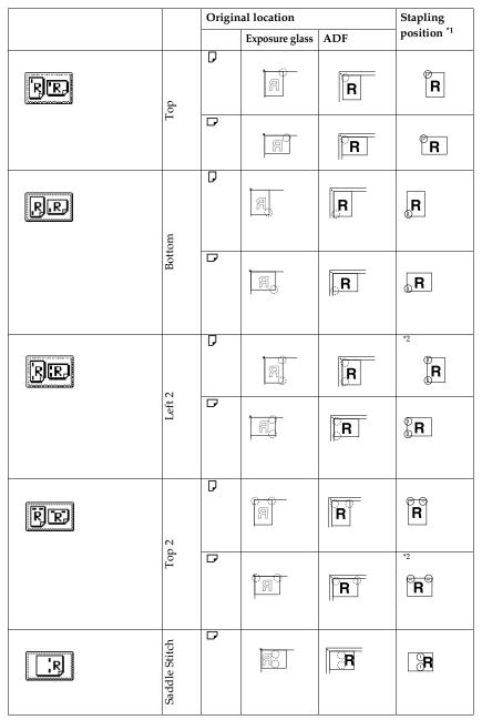
This table shows the stapling positions, not the orientation of delivery. Not available for A3, B4 JIS or  $11" \times 17"$ ,  $8^1/_2" \times 14"$  size paper. \*1
