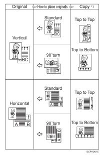
\*1 This table shows the orientation of images on the front and back of copies, not the orientation of delivered copies.
