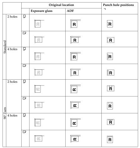
$^{\ast 1}$   $\,$  This table shows the punch hole positions, not the orientation of delivery.
