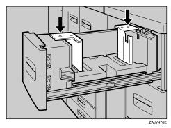
**4** Fasten the side fence with the screws.
