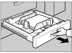
Press the lock button, and then adjust the back and side fences to the new paper size while pushing the release lever.
