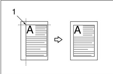
**1. Point where the machine starts scanning.**
