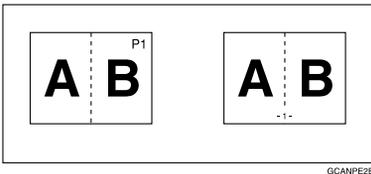
If you combine this function with the Duplex (Top to Top) function and select the "P1, P2" or "1/n, 2/n" format, page numbers on the back are printed as follows:
