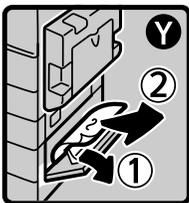
1. Open the lower right cover of the optional paper tray unit and remove the misfed paper.
