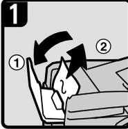
1. Open the ARDF cover, and then remove the misfed original.
