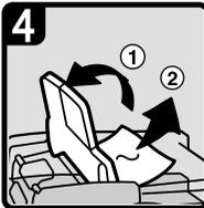
4. If you cannot remove the misfed original, open the ARDF external cover, and then remove the misfed original.
