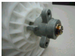
NG setting (Boss is not set in the dent of the gear)
