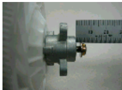
NG setting (Boss is not set in the dent of the gear)
