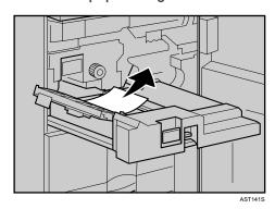
After removing the paper, return the lever and the unit to their original positions.
