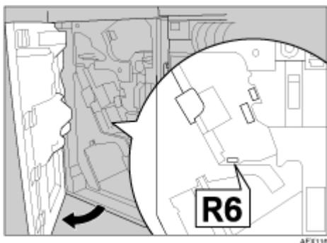
After removing the paper, return the lever to its original position.
