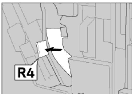
After removing the paper, return the lever to its original position.
