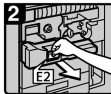
3. Pull handle E2 and fully pull out the duplex unit.
