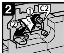
3. Turn lever C2 counter-clockwise and remove misfed paper.
