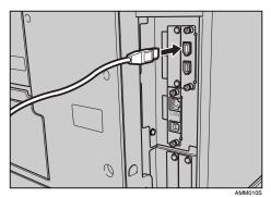
2 For IEEE 1394 (SCSI print) connection, plug the other end of the cable into the interface connector on the host computer.
