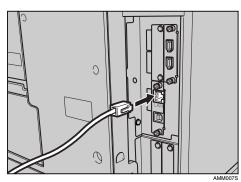
**4** Connect the other end of the Ethernet cable to a network connection device such as a hub.
