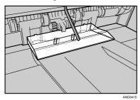
Close the front cover of the finisher. The Z-fold support tray is lowered to complete the installation.
