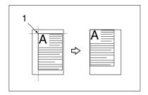
① Point from which the machine begins scanning
