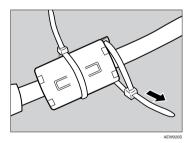
5. Attach the cable (ferrite core end) to the printer's parallel interface.
