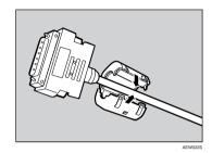
2. Fit one tie wrap snugly around the center of the ferrite core to prevent the core coming loose.
