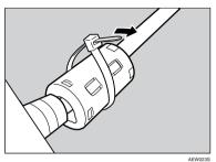
**4** Fit the other tie wrap snugly around the end of the ferrite core to prevent the core moving along the cable.
