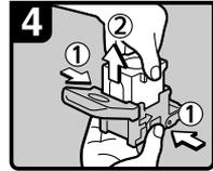
5. Holding both sides of the cartridge, pull up the upper unit.
