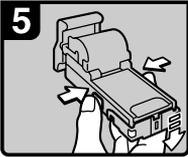
5. Push the buttons on both sides of the cartridge and open the face plate.
