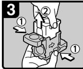
4. Holding both sides of the cartridge, pull up the upper unit.
