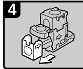
5. Remove the empty refill in the direction of the arrow.
