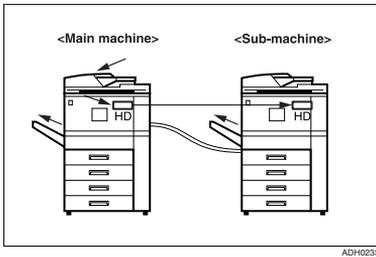
You can connect two machines together. When you set up a copy job on one machine (the main machine), data is transferred to the other (the sub-machine) so that copies can be made on both machines simultaneously (Connect Copy).
