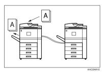
Using the idle machine as the main machine (Connect Copy)
