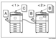
When machine <1> has finished with Original A, it begins copying Original C. If machine <1> finishes copying it allotment of Original C before machine <2> finishes with Original B, machine <1> will take over to copy the remainder of Original C.
