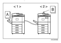
Machine <2> begins copying Original B. Machine <1> also starts copying Original B when it has finished with Original A.
