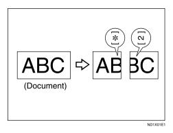
For example, this function splits the document if the document length is 20 mm (0.79") or longer than the paper used. The document is reduced if it is less than 20 mm (0.79"). When a document is split, an asterisk ( $\frac{\textbf{X}}{\textbf{X}}$ ) is inserted at the split position and about 10 mm (0.39") of the split area is duplicated on the top of the second sheet.
