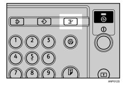
The interrupt key indicator lights. The machine stops scanning.
