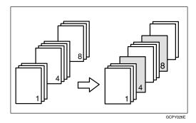
• Print on front side only Prints on the front side of slip sheets even if duplex printing is selected.
