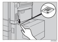
When the key stops blinking and lights up, open the top cover.
