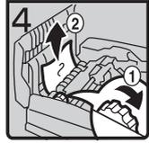
4. If you cannot remove the misfed original, turn the dial ① clockwise and remove the misfed original ②.
