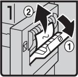
1. Open the side cover of duplex unit and remove misfed paper.
