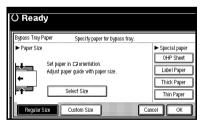
3 Enter the vertical size of the paper using the number keys, and then press [#]. 4 Enter the horizontal size of the paper using the number keys, and then press [#].
