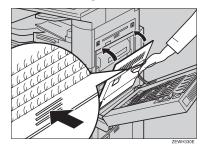
**6** If the duplex unit is installed, close the duplex unit.
