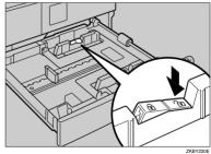
5 While pressing the release lever, adjust the side fences.
