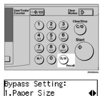
Press the (b) key to select "2. Paper Type", and then press the [OK] key.
