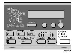
☐ Press the [Original Type] key to step through the following types:
