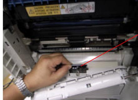
7) Reinstall the "Guide Plate - Manual Feed" [D] using a short Phillips screwdriver. (2 screws [E])
