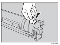
**5** Insert the toner cartridge and make sure it locks securely into place.
