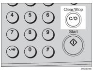
The machine will stop storing the data from the original and the data will not be sent.
