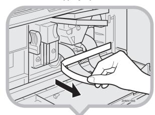
**9.**Push the lever (①) and pull out the toner cartridge holding ① and ②.
