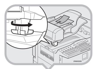
3. Pull the fixing material to the right to remove.
