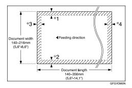
The part shaded will not be scanned, because it is outside the maximum scanning width range.
