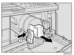
**5** Take the cord off the hook and remove the connector.
