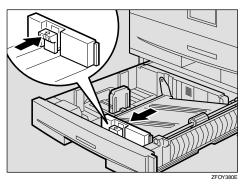
**4** Push the metal plate down, and then square the paper and load it in the tray.
