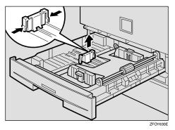
**3** While pressing the release lever, adjust the side fences to the desired paper size.
