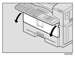
Push the lever (1) and pull out the toner cartridge holding (1) and (2).
