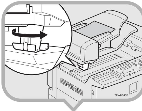
3. Remove the fixing material to the right.
