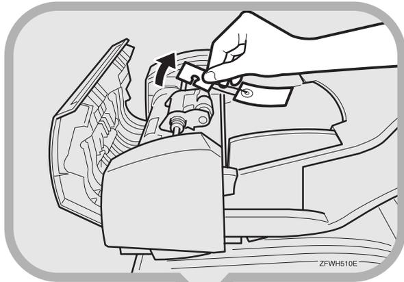
**8. Remove the fixing material.**
